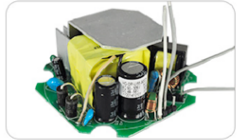
Power Supply (Rubycon capacitor)
