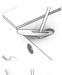
Step 3- Using the shorter aircraft! cable (with two tabs on both ends),! insert the two slot-shaped tabs into! the slots on both sides. This!is accomplished by first inserting!one end of the tab and using the slot!to move the cable as desired to bring in the second end of the tab.!Once this tab has been inserted!into the luminaire, it will be safely!secured into place for mounting.
