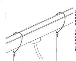
Step 1- Wrap two pieces of cables across a ceiling beam and extend down to the required mounting height.
