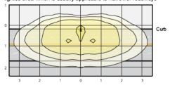
TYPE III placed on the side of the roadway or edge of the area to be lighted. It produces an oval-shaped lighted area and is usually applicable to medium width roadways
